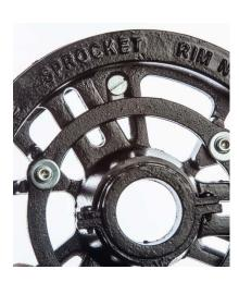
3. Place the chainwheel against the front of the valve hand wheel aligning the slots of the hammer blow attachment to the holes in the plate. Put one washer (if included) on a bolt, pass the bolts through the top slot in the hammer blow attachment from the front, and through the holes in the plate. Loosely secure with a washer (if included) and nut.
